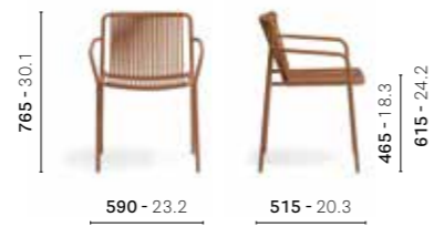
3665 Armchair, steel frame, PVC flexible profile seat and backrest
